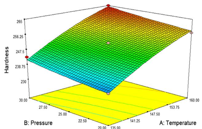
**Fig. 7** 3D plot of hardness as a function of temperature and pressure.
