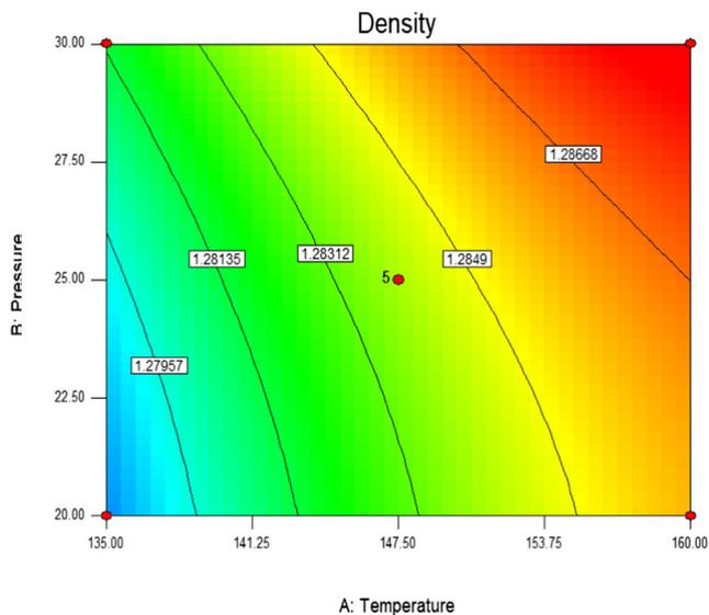
**Fig. 2** Contour plot of density as a function of temperature and pressure
