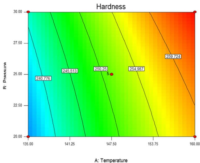
**Fig. 6** Plot of hardness as a function of pressure and temperature
