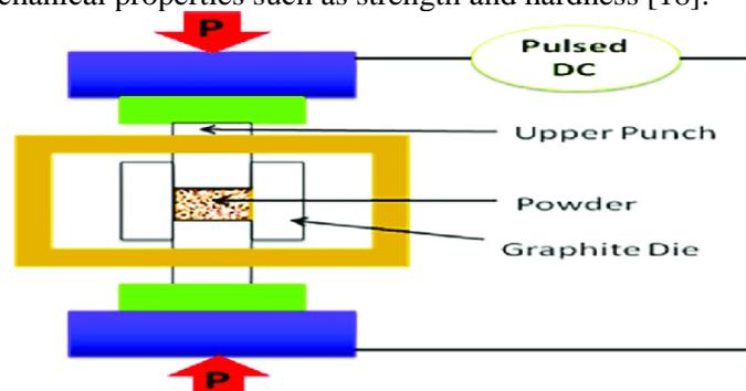
**Figure 1: Schematic diagram of spark plasma sintering technique [23]**
